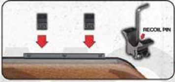
2 Attach ring mounts to base of rifle. The rear ring mount requires the installation of the recoil pin to prevent the rings from moving or slipping on the receiver grooves or rail. Lower the recoil pin down less than ¼" (0,6 cm) into the ring perforation.
