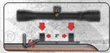
3 Minimum distance between mounts 2" (5cm) Tighten the horizontal screws in the lower half of the rings. Place scope onto the bottom half of the ring mounts.
